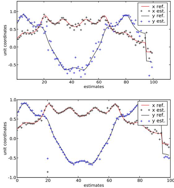
**Fig. 2** Estimation results for  $k$ -means (top plot) and RANSAC (bottom plot), for synthetic flow, 30% outliers and 0.001 Gaussian noise (reference signal is the normalised true translation from the simulation) Note the significantly better performance of the RANSAC algorithm due to the Newton iteration step.
