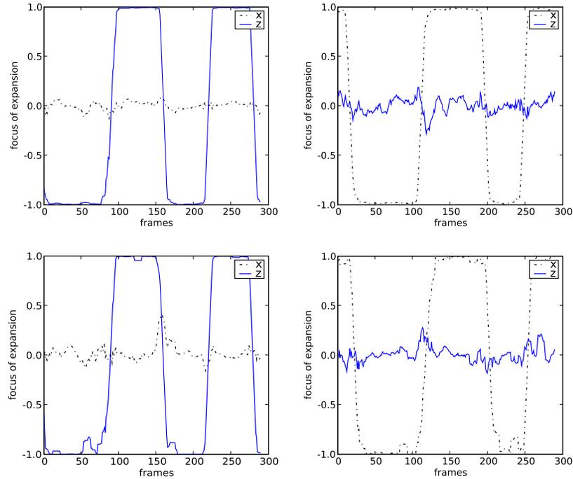
**Fig. 4** FoE extraction for a camera mounted on a linear rail. The plots on the left show the results for the camera moving forwards and backwards along the optical axis (top:  $k$ -means, bottom: RANSAC), the plots on the right for the camera moving sideways perpendicular to the optical axis (again top:  $k$ -means, bottom: RANSAC).
