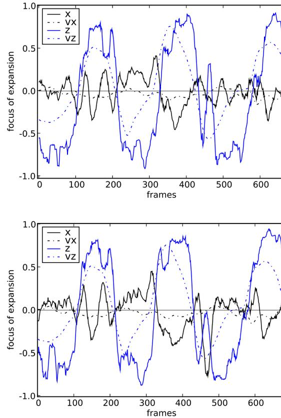
**Fig. 5** FoE extraction for real world flyer scenarios, flying forwards and backwards along a straight line. The plot on the top shows the estimates from  $k$ -means, the lower plot shows the RANSAC results. The dashed lines are the approximate velocity data integrated from the inertial unit. Note that the FoE estimates are normalised, the velocity is not.
