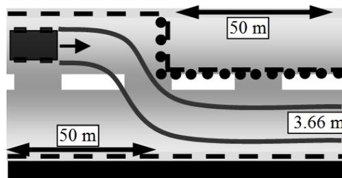
Multiple hazard avoidance experiments tested the controller's ability to navigate more complex road/hazard setups that required maneuvers with appreciable load transfer. In these tests (illustrated in Fig. 8), both lanes of travel were blocked at different locations, forcing the vehicle to change lanes to avoid the first hazard, then change lanes again to avoid the second as in a double-lane-change maneuver.
