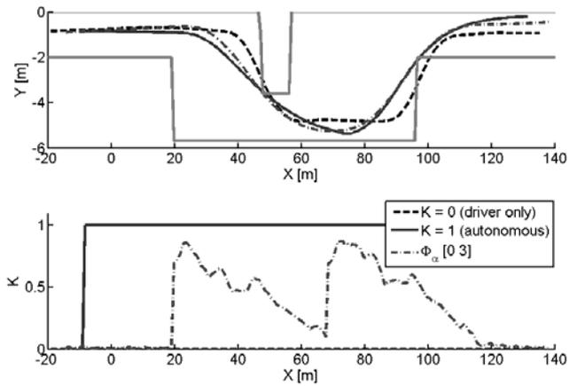
As Fig. 12 shows, intervention by the semi-autonomous controller slightly preceded an otherwise-late driver reaction. The combined effect of both inputs was then sufficient to avoid both road hazards.
