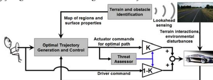
Fig. 1 Diagram of an active safety system
